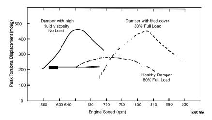
Fig. 10. The effect of viscous damper faults on the 2.5 order response curve of a 16 -cylinder "V" engine driving a generator (derived from service failure records)
