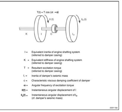
Fig. 3. A two-mass dynamic model of an engine installation fitted with a viscous shear torsional vibration damper
