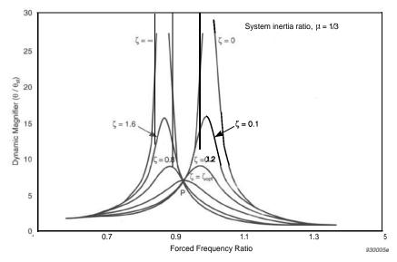
Fig. 4. Viscous damper: Dynamic magnifier curves for various values of damping ratio ( $\zeta$ )
